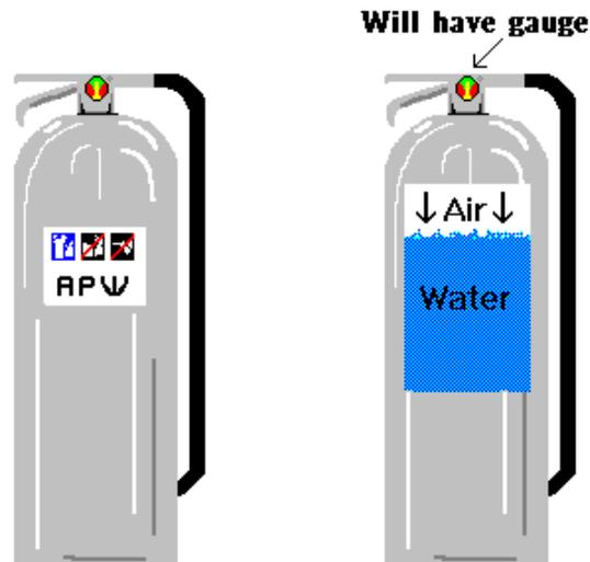
APW's extinguish fire by taking away the “Heat” element of the Fire Triangle.
