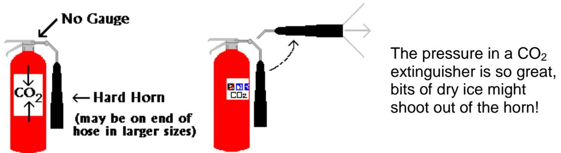
CO<sub>2</sub> cylinders are red. They range in size from 5 pounds to 100 pounds or larger. On larger sizes, the horn will be at the end of a long, flexible hose.
